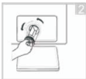
Open the filter by turning it counter clockwise
